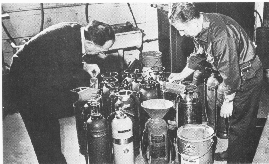
"FILL IT UP" — A MUST FOR FIRE EXTINGUISHERS. Anthony Crispino and Bert Lafrenier of our Fire Dept., keep all extinguishers ready for action, except the carbon dioxide type which is a gas type requiring special equipment to refill.
